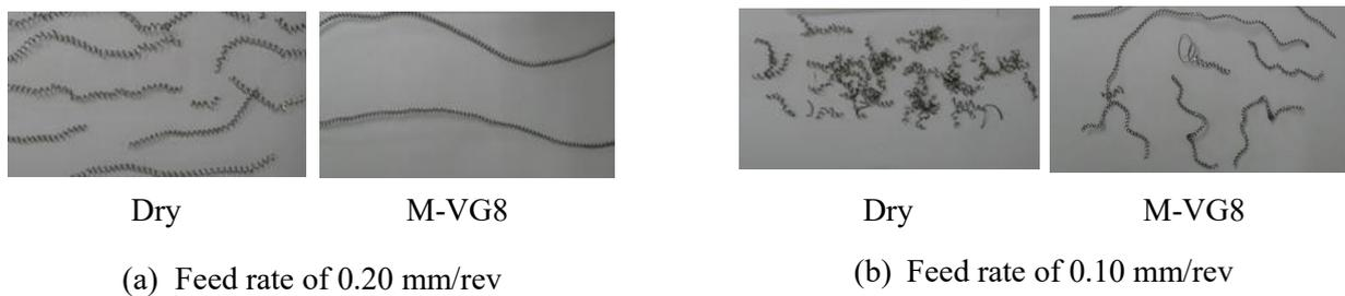
**Fig. 2.35** Difference of chips shape in cutting fluids when turning SUS304 at the cutting speed of 10 m/min
