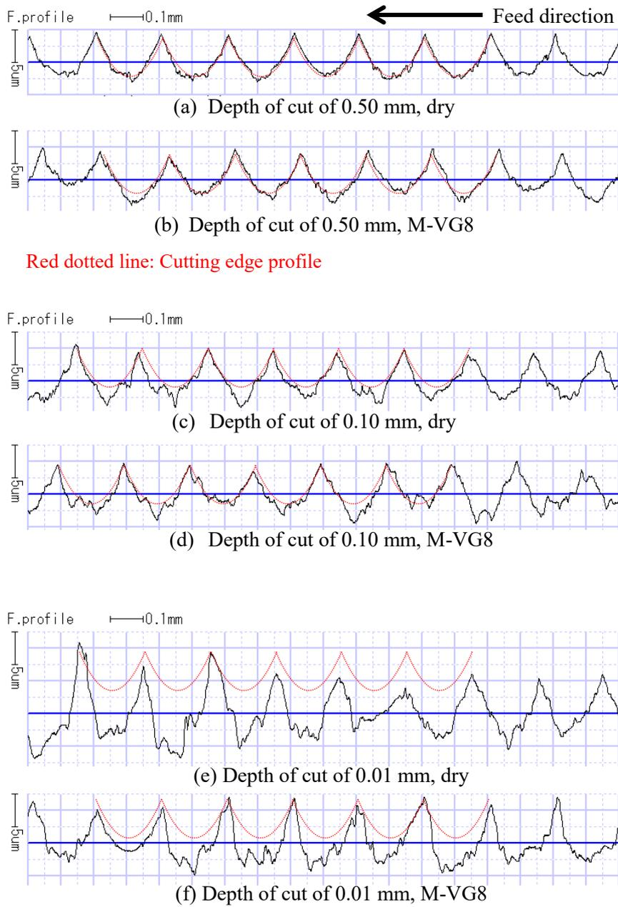
**Fig. 2.43** Difference of surface roughness curve in depth of cut when turning SCM435
