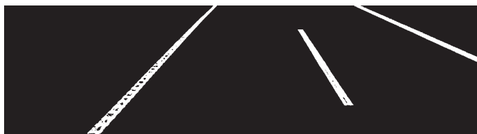
(b) Binarization result of extracted road surface region
