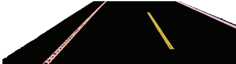
(a) Binarization result of extracted road surface region. Each line is indicated by a different color
