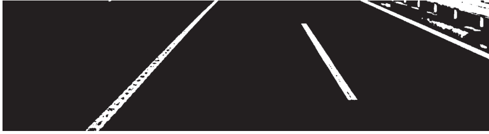
(b) The result of lane mark detection using ROI
