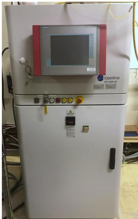
Fig. 3.3 Diode laser oscillator.
