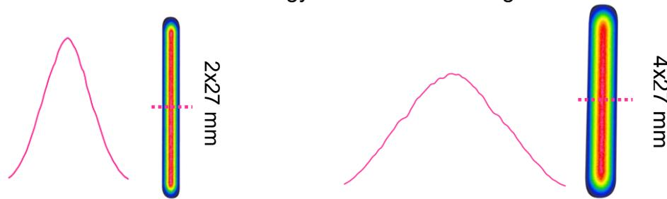
Fig. 3.13 Laser beam profile.
