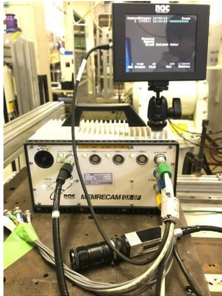
Fig. 3.5 High-speed camera equipment.
