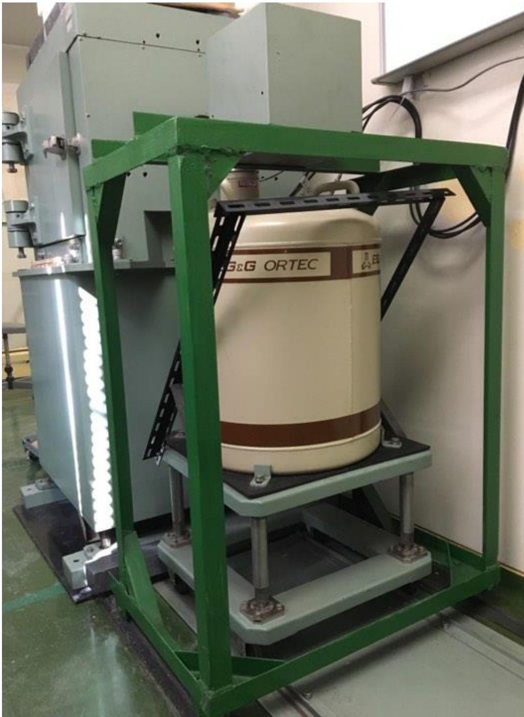
Fig. II-6: Gamma measurement system (COAX) in Hiroshima University
