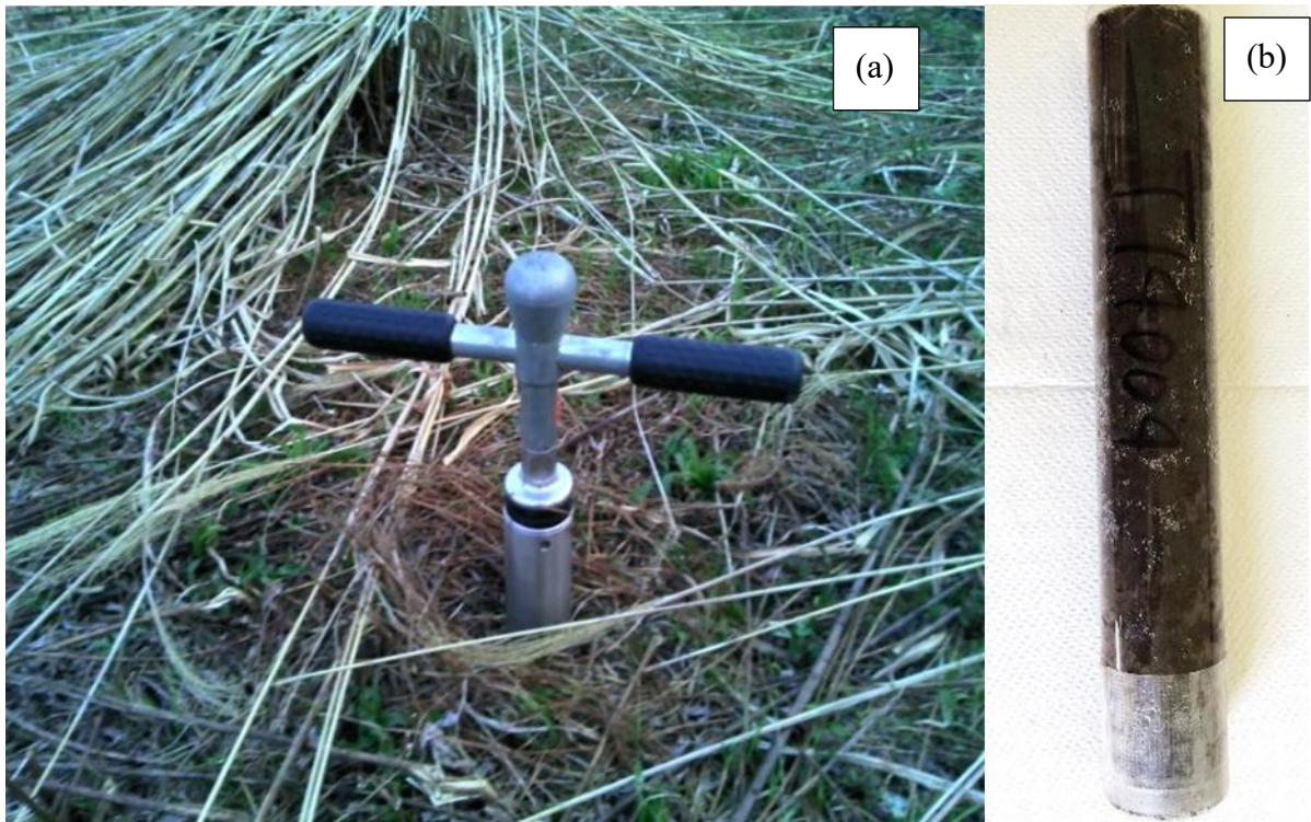
Fig. II-2: Soil core sampling method – (a): Sampler - (DIK-110C, Daiki Rika Kogyo Co., Ltd.); (b): 30 cm soil core
