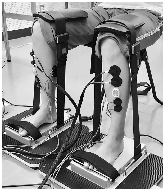
Figure 1 Illustration of each subject sat in a chair with their knee flexed at a 90^\circ angle, while the bases of the metatarsals were held in place with a stabilizing belt.
