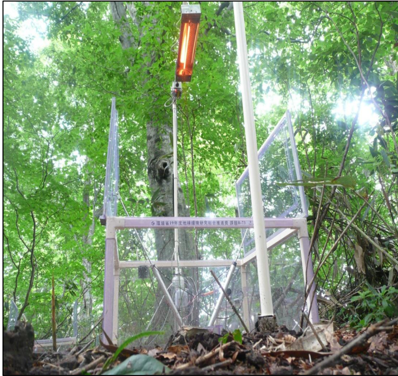
Fig. 3-1 The automatic open top chamber
