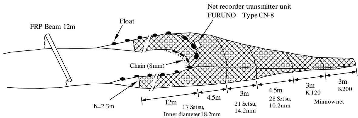
**Fig. II-1-2.** Diagram of a midwater beam trawl net to collect whitespotted conger leptocephali in the northeastern Harima Nada Sea.
