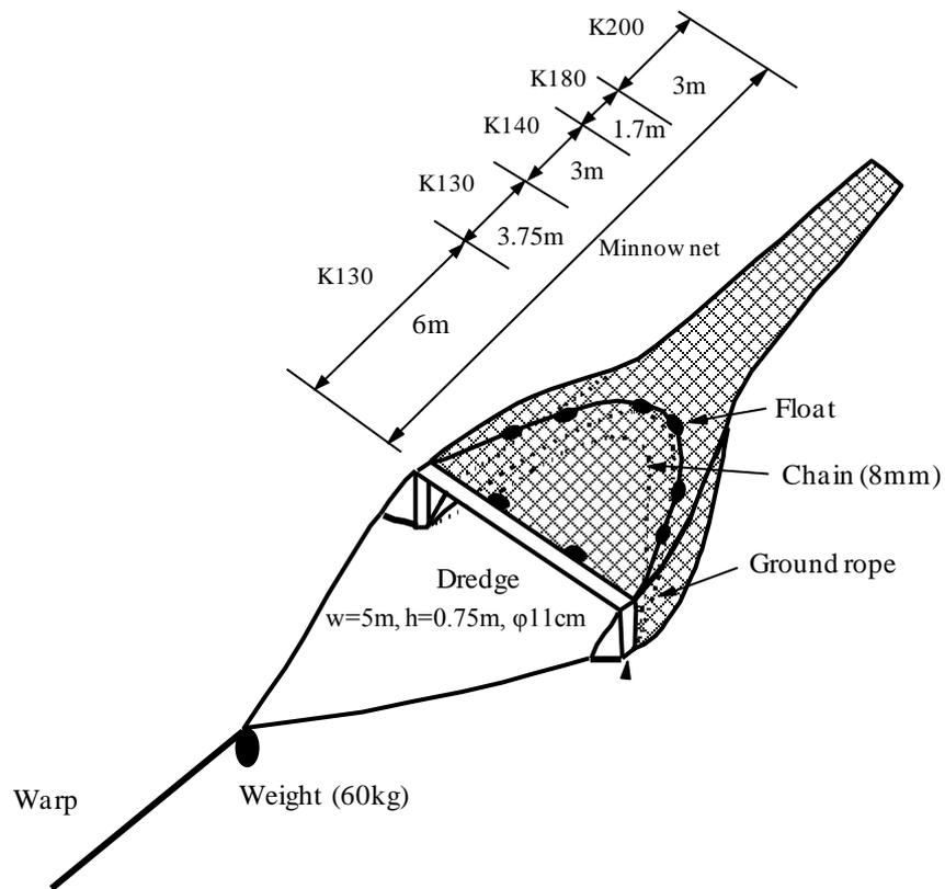
**Fig. III-2.** Diagram of a bottom trawl net to collect newly settled whitespotted conger in the northeastern Harima Nada Sea.
