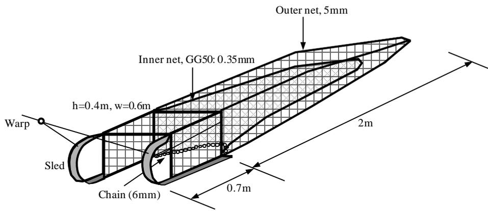
**Fig. III-4.** Diagram of a sledge net used to collect epifaunal benthos in the northeastern Harima Nada Sea.
