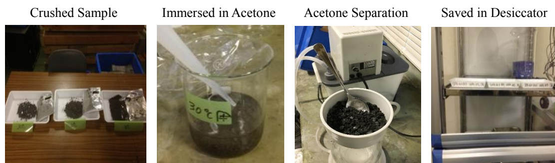
Figure 3-9 Hydration Stop Operation of Cement Paste
