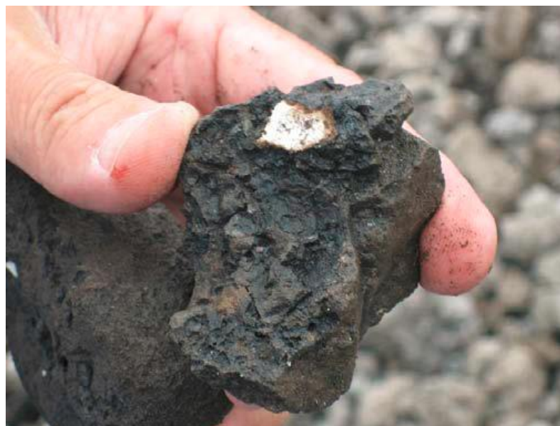
Figure 2- 3 Free lime pocket inside a gravel-size steel slag aggregate (Yildirim and Prezzi, 2009).
