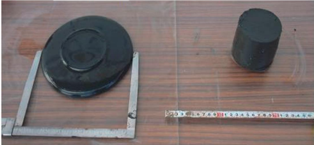
Figure 2- 11 Physical state of dredged marine soil before (left) and after (right) mixing with BOF slag (Yamagoshi et al., 2014a).
