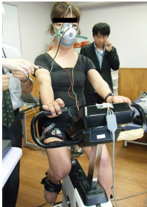
Figure 2-6. Measurement of cardio-respiratory function using a cycle ergometer in 2009. In 2003, it was impossible to measure a cardiorespiratory function of the subject, due to weakness of muscle strength.
