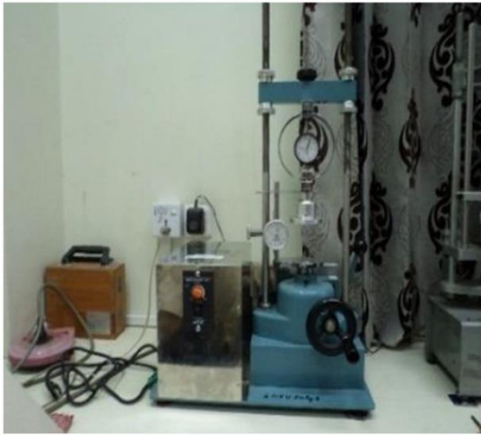
Figure 4-23 Unconfined Compression Test Machine
