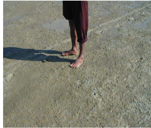
Photo - 5.4 Riverbed conditions at Thilawa Port Area (People can easily walk on the riverbed at some area at Thilawa due to thin firm clay layer (Thickness \leq 0.3 \sim 0.5\text{m} ) at riverbed in Thilawa)
