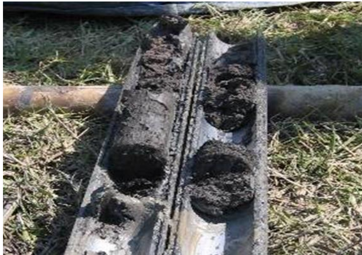
Photo - 5.6 Soft clay (Clay-II, equivalent to AC-I Layer in Sub-areas in Yangon) at Thilawa
