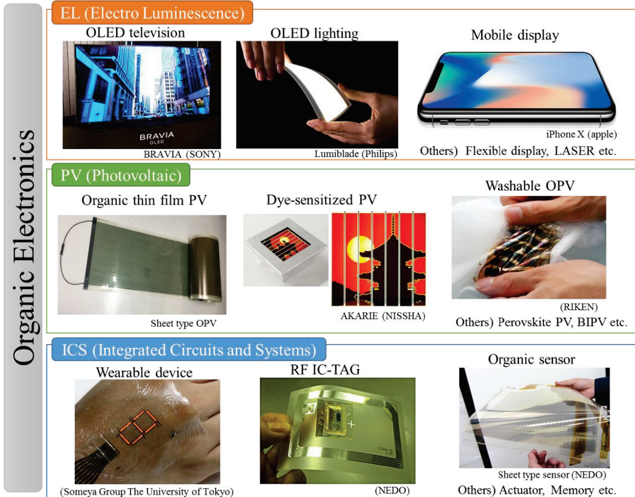
Fig. 1-2: The product examples of organic electronics with three categories: Electro Luminescence, Photovoltaic, and Integrated Circuits and System. [15-21]
