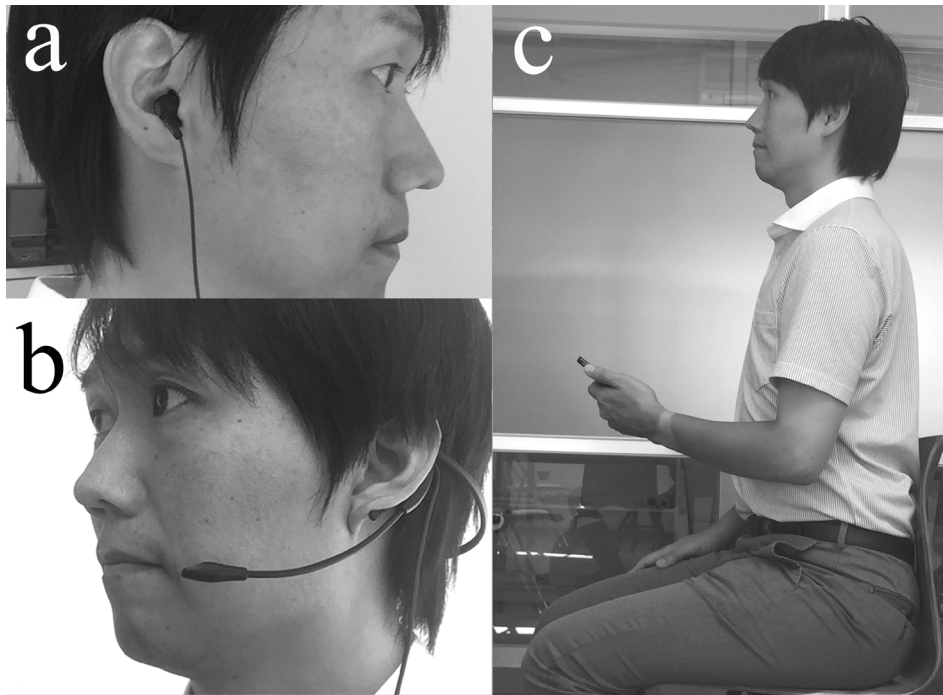
Figure 3.1 Types of microphones and measurement position. (a) In-ear microphone. (b) Mini speech microphone. (c) Smartphone microphone.
