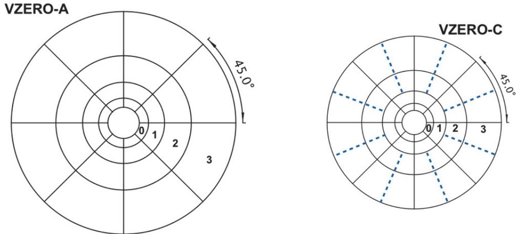
Figure 16: Sketches of V0A and V0C arrays [48].
