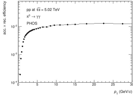
Figure 152: The acceptance  $\times$  reconstruction efficiency of  $\pi^0$
