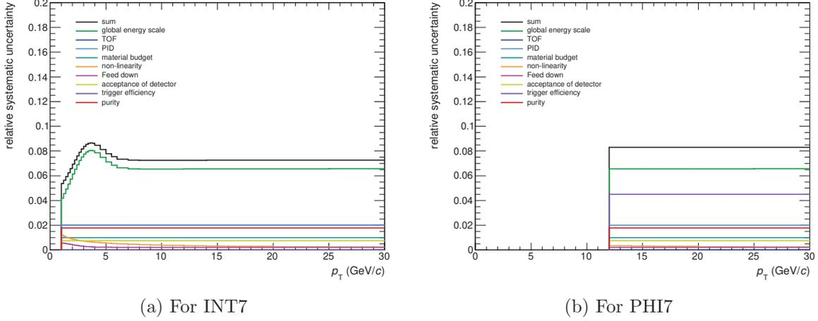
Figure 131: Systematic uncertainties for  $\gamma^{\text{inc}}$  in Pb–Pb collisions at  $\sqrt{s_{\text{NN}}} = 5.02$  TeV for centrality 0-10%.
