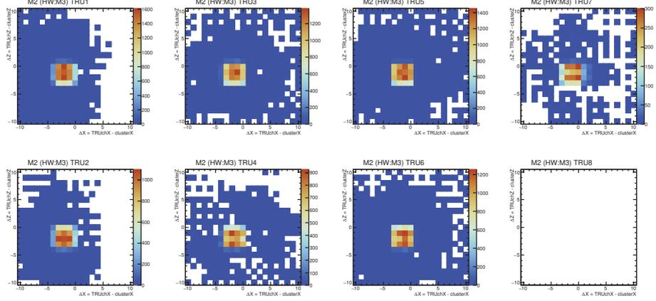
(b) The distance between fired TRU channels and cluster position on M2 in LHC15n.
