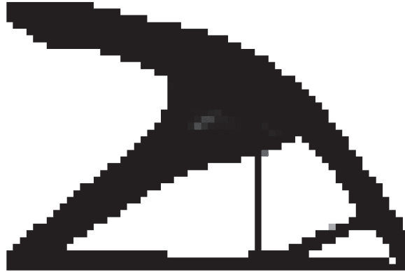
Figure 28 Checkbording limitation using 8 nodes element (60x40 elements)
