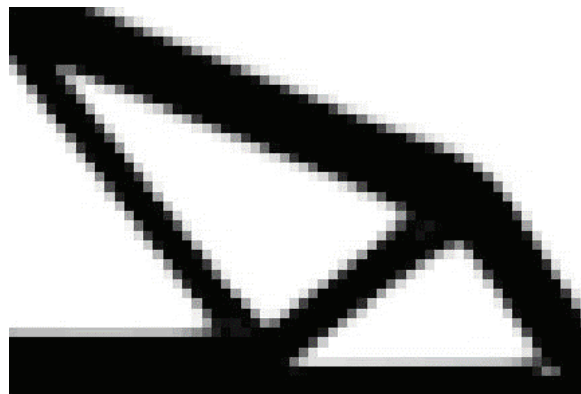
Figure 31 Checkboard limitation using 4 nodes element (60x40 elements)
