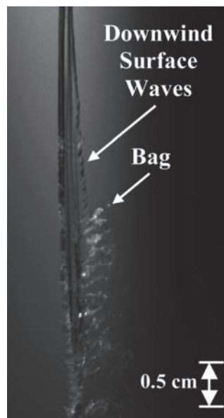
Figure 1.11 Downwind surface waves of round non-turbulent liquid jets in uniform gaseous crossflow within the bag breakup regime.
