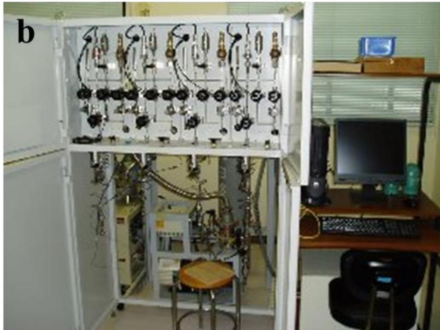
**Figure 3.7: (a) Schematic of Sievert's type measurement, (b)PCI equipment**
