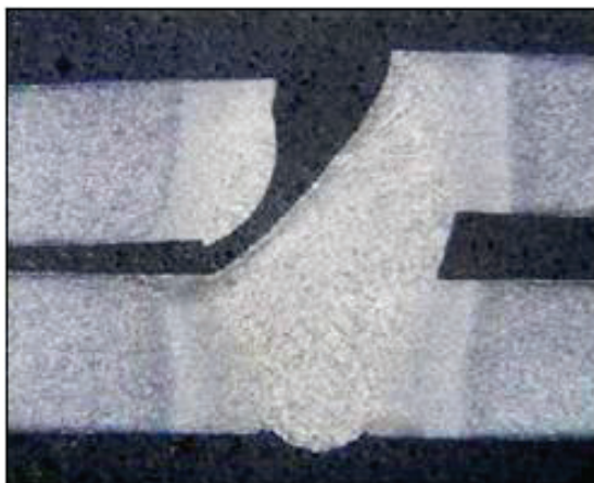
Fig. 1-4 Weld defect example on cross-section of laser welded lap joint with large gap between steel sheets 10) .
