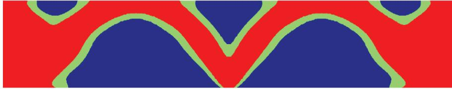
Fig. 4.17 Robust optimal design of the two-edge clamped beam for maximizing the frequency gap between the second and third frequencies.
