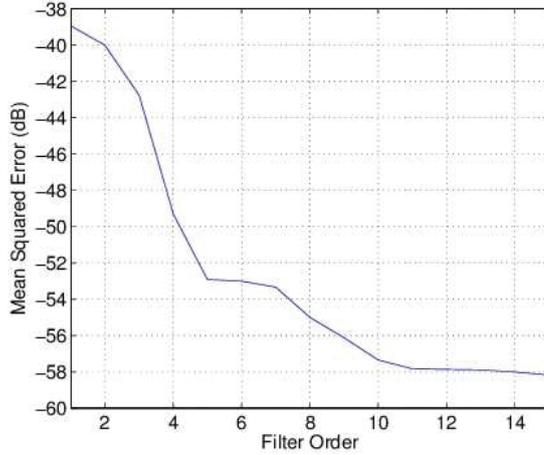
Figure 4.2: MSE of optimal FIR noise shaping filters as a function of their order.
