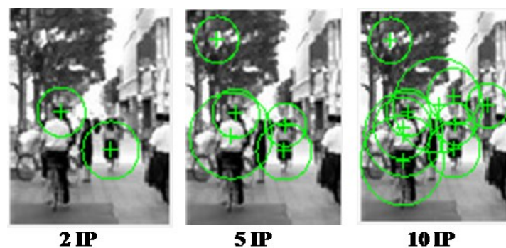
Fig.2. 1 An illustration of selection results of the original SURF algorithm with different numbers (2, 5, 10, respectively) of interest points (IP).
