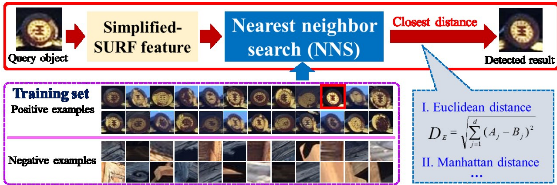
Fig.5. 3 The flowchart of the object detection system employing the NNS classifier.
