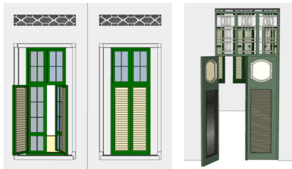
Figure 4.3 Louver windows and ventilation openings above windows/door.
