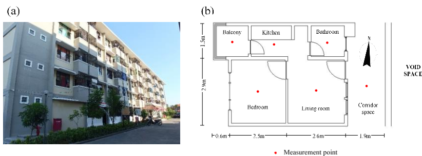
Figure 3.7. (a) View of selected new public apartment and (b) floor plan of selected unit.
