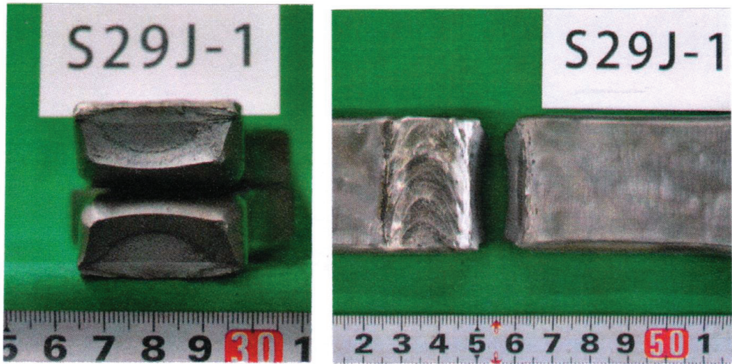
Fig.4.3.3 Fracture surface and pass after fatigue test (S29J-1, 350 N/mm 2 , 3.15 × 10 5 cycles)
