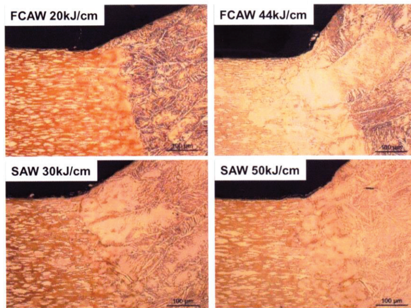
Fig.3.5.3 Results of microscopic test of welded section for butt welded joints [Fusion line] (SUS329J3L-Clad)
