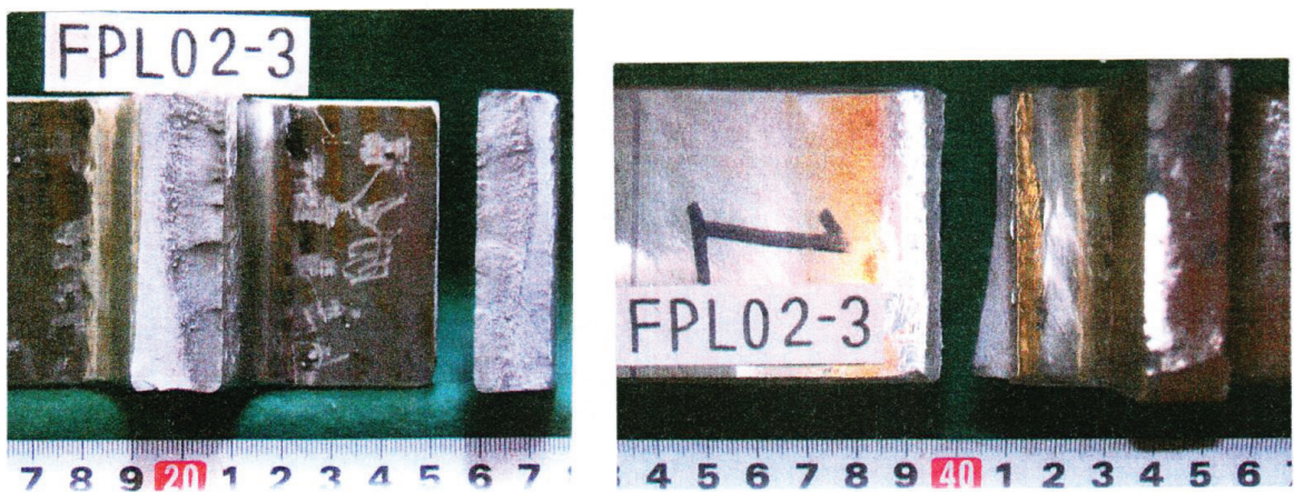
Fig.4.4.4 Fracture surface and pass after fatigue test (FPL02-3, 398 N/mm 2 , 1.38 × 10 5 cycles)
