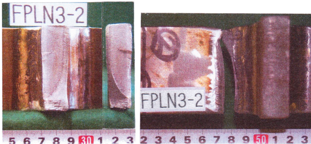
Fig.4.5.10 Fracture surface and pass after fatigue test (FPLN3-2, 200 N/mm 2 , 1.09 × 10 6 cycles)
