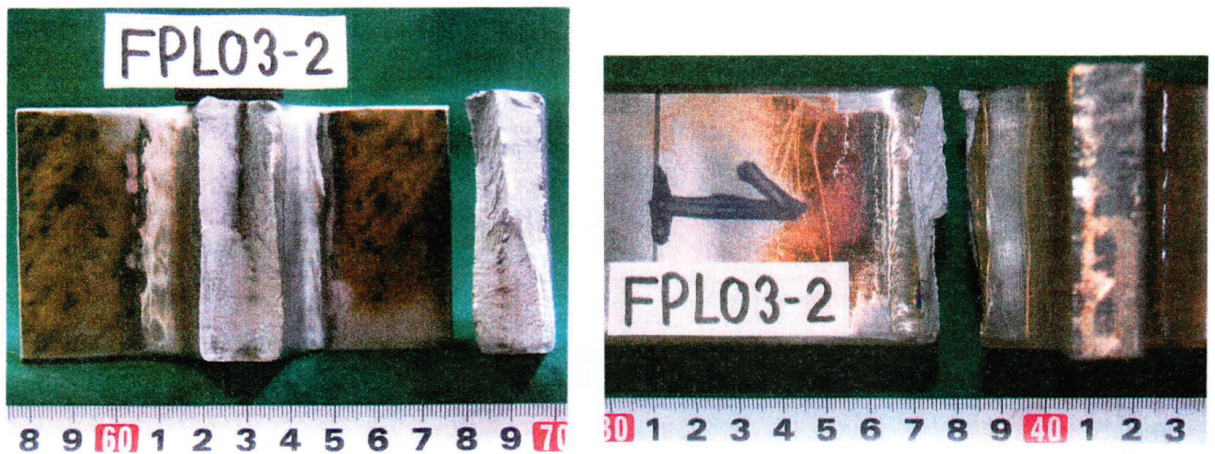
Fig.4.4.6 Fracture surface and pass after fatigue test (FPL03-2, 350 N/mm 2 , 3.60 × 10 5 cycles)
