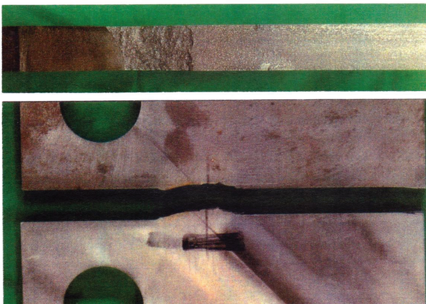
Fig.2.3.10 Fracture surface and pass after fracture toughness test (FTI-2, -144^{\circ}\text{C} )
