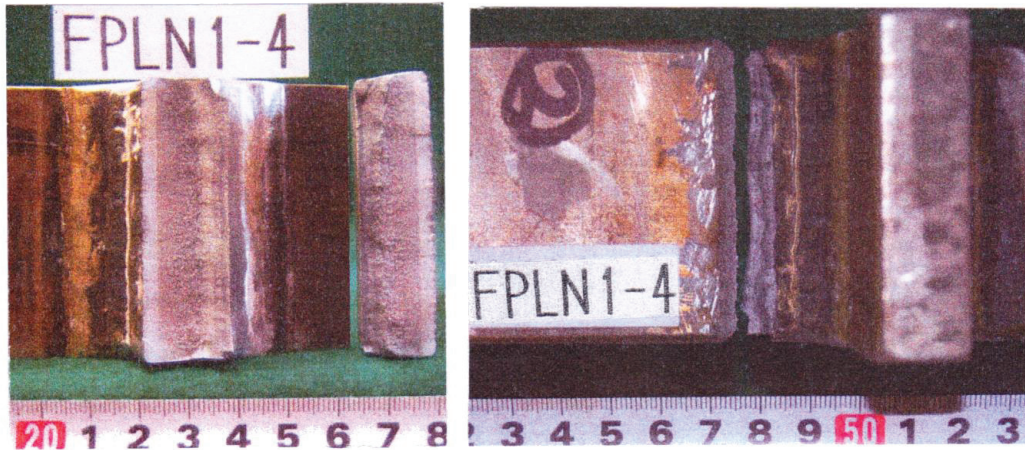
Fig.4.5.9 Fracture surface and pass after fatigue test (FPLN1-4, 250 N/mm 2 , 1.66 × 10 5 cycles)
