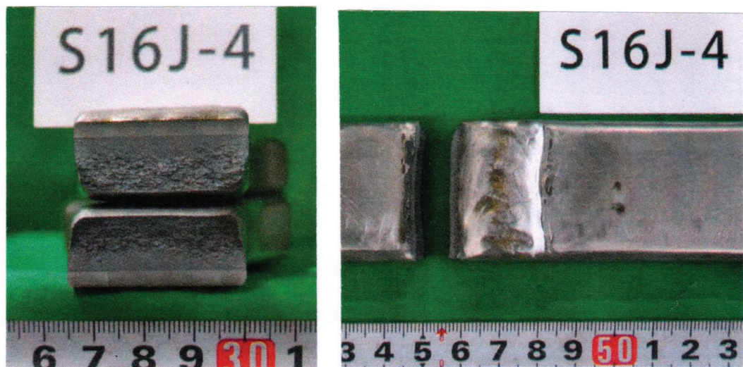
Fig.4.3.4 Fracture surface and pass after fatigue test (S16J-4, 200 N/mm 2 , 1.26 × 10 5 cycles)
