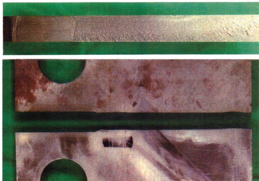
Fig.2.3.12 Fracture surface and pass after fracture toughness test (FTI-4, -159^{\circ}\text{C} )
