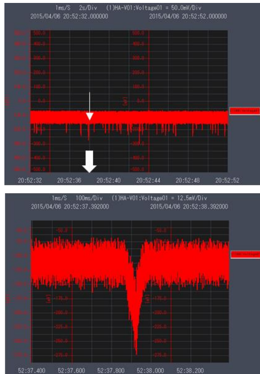
Figure 3-27 Signal when using a long-pass filter
