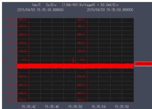
Figure 3-26 Background noise when using long-pass and band-pass filters
