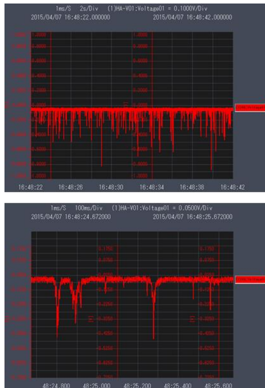
Figure 3-31 Effect of the optical slit on the signal
