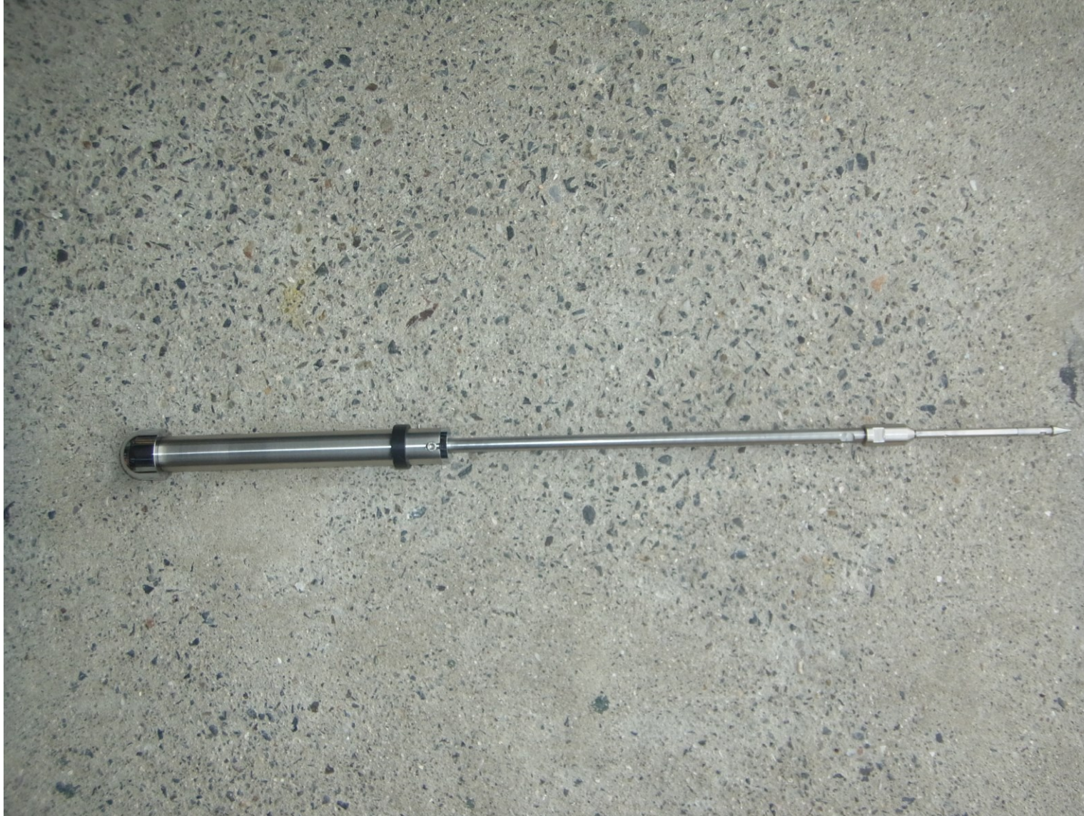
Appendix 4. Device for measuring penetration resistance with corn and spring.
