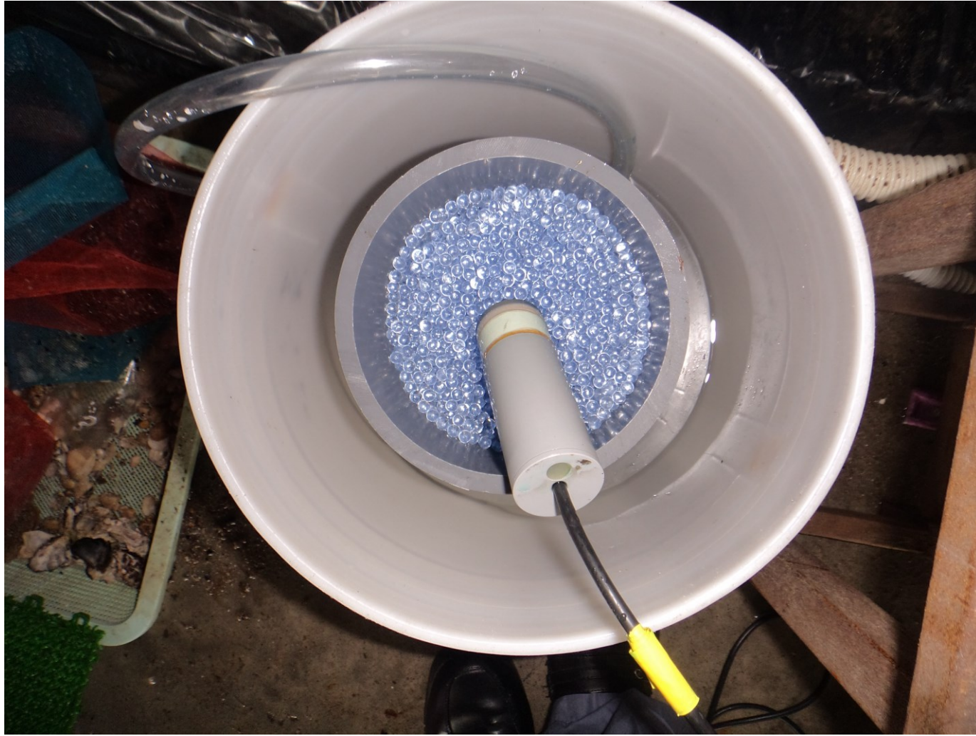
Appendix 8. Experimental column with glass beads and suction meter.
