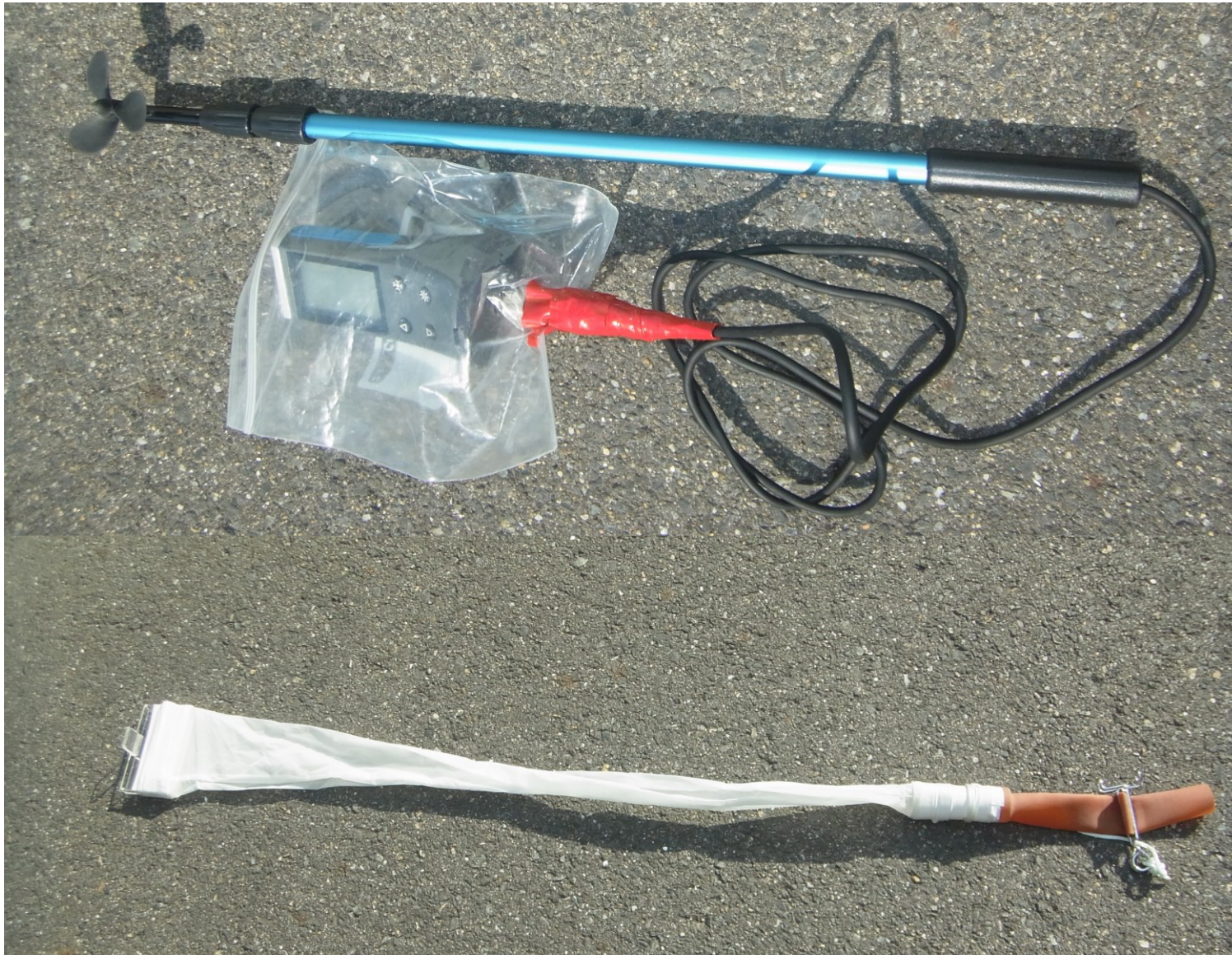
Appendix 7. FLOWATCH, device for measurement of current speed (upper). Sand trap for drift with 63 \mu m mesh (lower).
