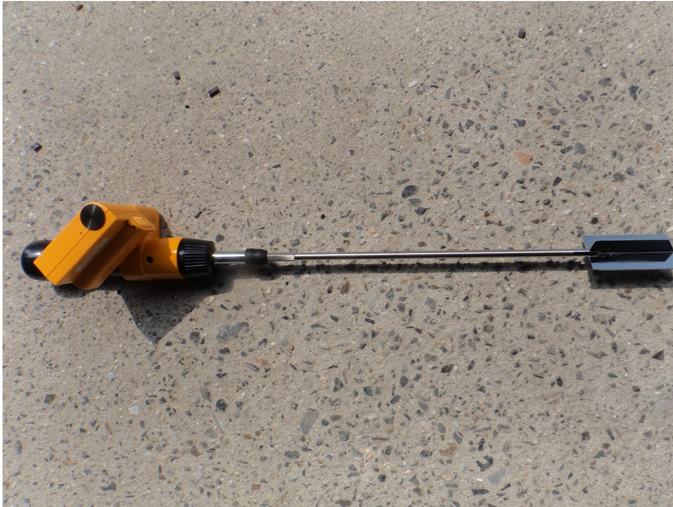
Appendix 10. Devices for measurement of deep vane shearing.
