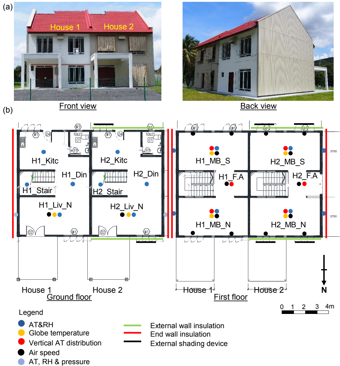
Figure 6.1. (a) Exterior views of the experimental houses (b) The floor plans of the experimental houses and the location of the measurement equipment.
