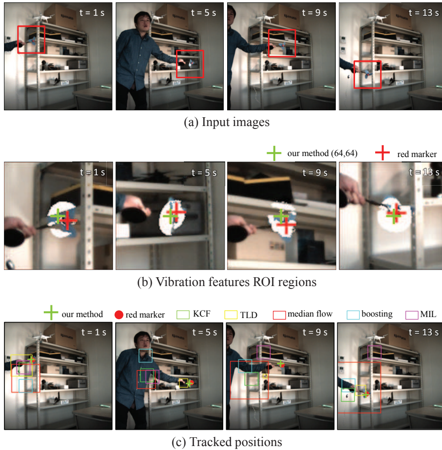
Figure 5.12: Input images of 512 \times 512 pixels, masked vibration features in the tracked ROI regions of 128 \times 128 pixels, and tracked results for single-object tracking methods in indoor scene experiment.
