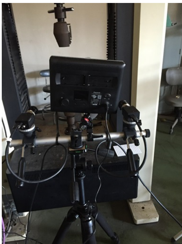
Fig. 5.16: Devices of digital image correlation.
