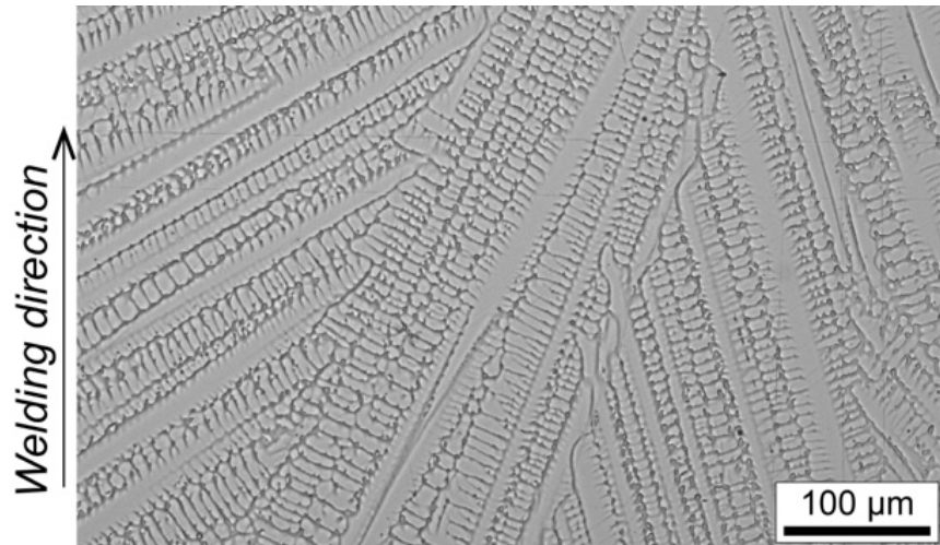
Fig. 23 Microstructure on weld bead surface during arc welding.
