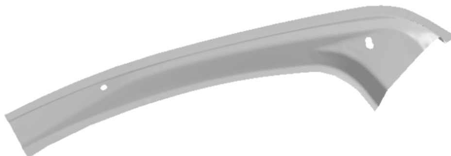
Fig. 4-2 Shape of front pillar reinforcement
