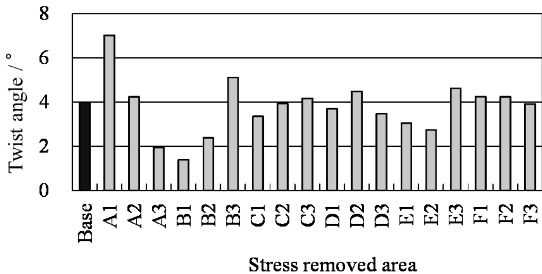
Fig. 5-12 Twist springback angles calculated by developed springback-root-cause analysis using stresses of zero in one of 18 areas, A1 to F3, and using stresses as shown in Fig.5-7 in other 17 areas compared with base twist angle of 3.9°
