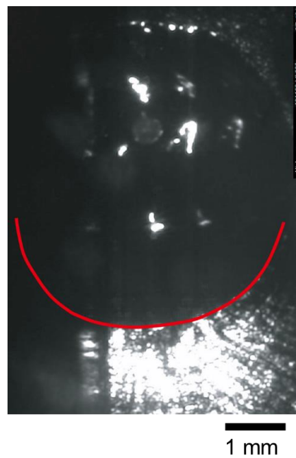
Fig. 3.8 In-situ observation image of the molten pool after Trans-Varestraint test during LBW at welding speed of 0.2 m/min under augmented strain of 4.3 %
