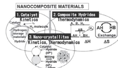
Fig. 2. Design concept of nanocomposite materials for hydrogen storage ( $\Delta\text{H}$ : enthalpy difference,  $\Delta\text{S}$ : entropy difference, AH, BH: hydride, The size of the hydrides: 10-100nm)
