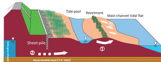
Groundwater flow formed around river structure (Groundwater flow occurred by water level difference with ①: tide pool, ②: delta groundwater (groundwater in inland area))
