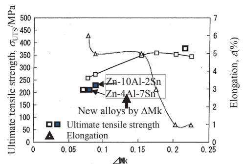
Fig.1 Relation between  $\Delta M_k$  and UTS, elongation.
