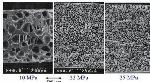
Fig. 2 Foaming of polystyrene using N<sub>2</sub>.
