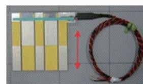
1 axis shear force sensor of 50mm square
