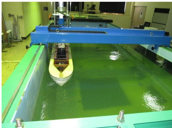
Photo.15 Drift angle test with changing the position for S-Cb81 ( $\beta=0\text{deg}, y_C=0.75\text{m}$ )
