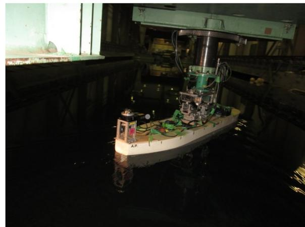
Photo.30 CMT in the towing tank for S-Cb81 ( $\beta=+10\text{deg}, r'=0.1$ )
