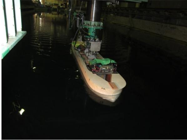
Photo.31 CMT in the towing tank for S-Cb87 ( $\beta=0\text{deg}$ )
