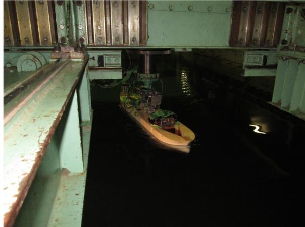
Photo.28 CMT in the towing tank for S-Cb81 ( $\beta=-10\text{deg}$ )
