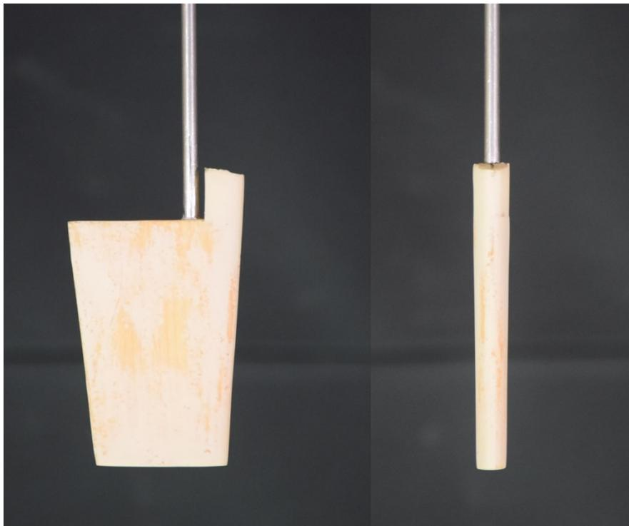
Photo.6 Model rudder for SR221(A)&(B)
