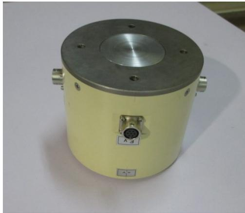
Photo.10 3-components load cell
