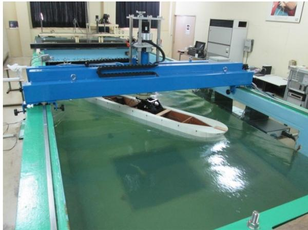
Photo.14 Drift angle test for S-Cb87 ( $\beta=-30\text{deg}$ )
