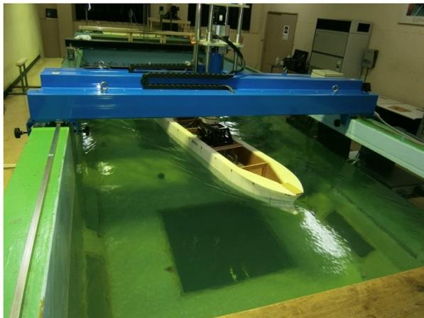
Photo.20 Drift angle test for SR221(A) ( $\beta=-12.5\text{deg}$ )
