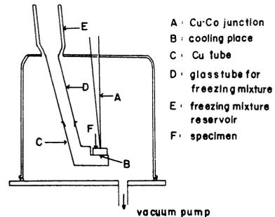
Fig. 1 Schematic diagram of low temperature replica apparatus
