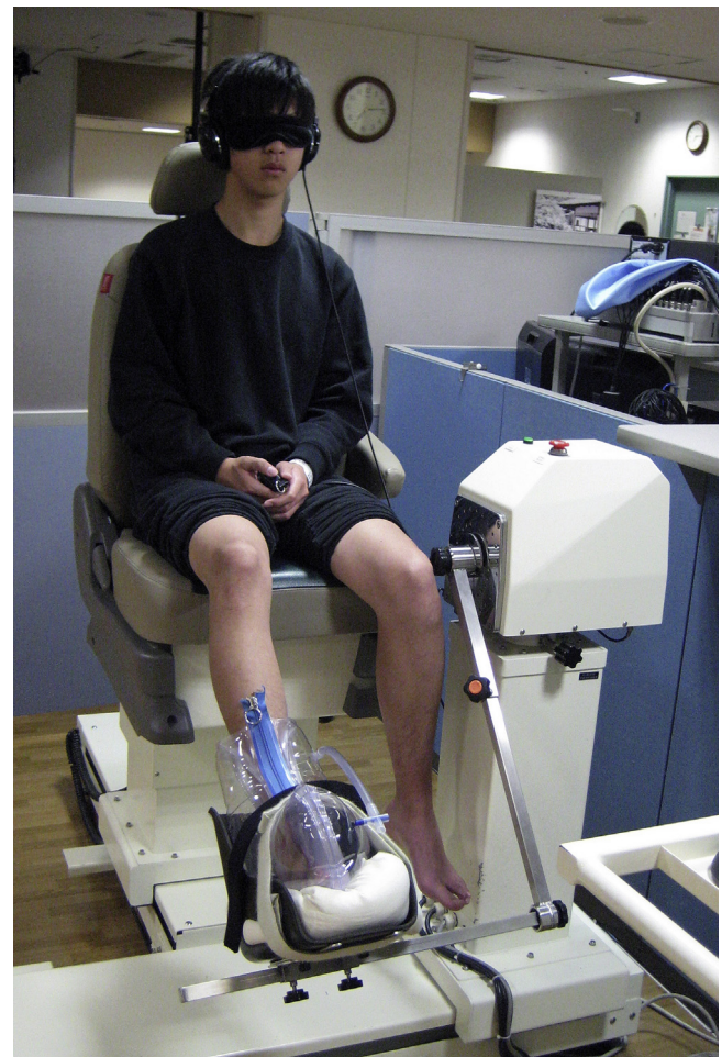
Fig. 3. Proprioceptive testing apparatus. Patients are tested in a seated position, blindfolded and have their ears covered to minimize visual and auditory cues. The testing limb is put into a pneumatic boot to keep the ankle in the neutral position and minimize cutaneous sensation. A hand-held switch enables each subject to stop the movement when they perceive it as joint motion.
