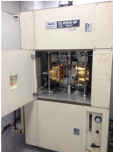
Fig 3.1 Floating Zone furnace for growing single crystal
