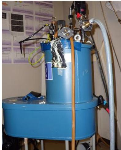
Fig. 2.1. The appearance of the superconducting magnet.
