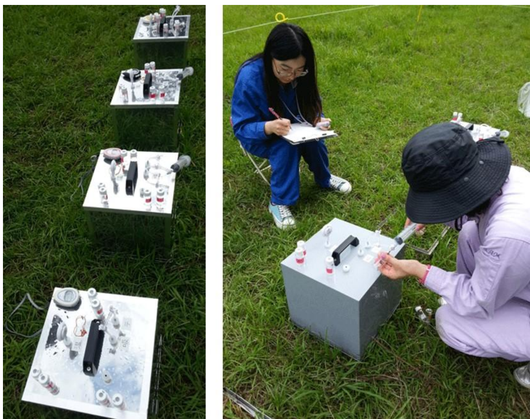
Figure 7.2 The equipment to measure greenhouse gas emissions.
