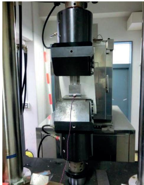
**Fig. 3.10** 200kN servo-hydraulic testing machine
