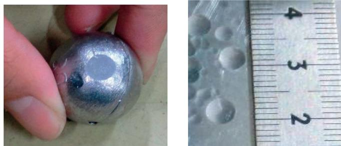
**Fig. 3.18** Deformation on the ball and surface of sensor
