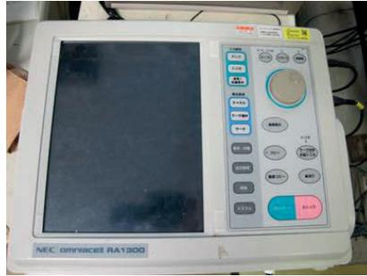
**Fig. 3.11** High-speed voltage recorder
