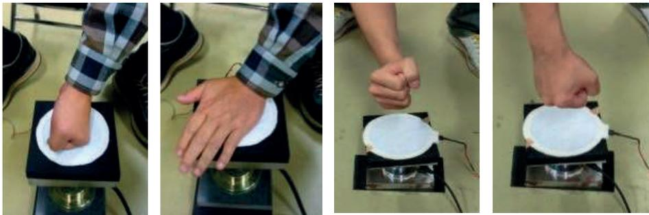
**Fig. 5.5** Fist press, palm press and fist punch of the sensor placed on the sponge rubber plate
