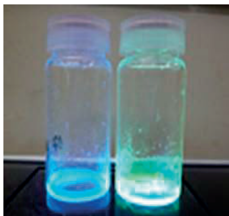
図 4.9 Digital photographs of the Sample 1(left) and Sample 5(right) under excitation at 350 nm.
