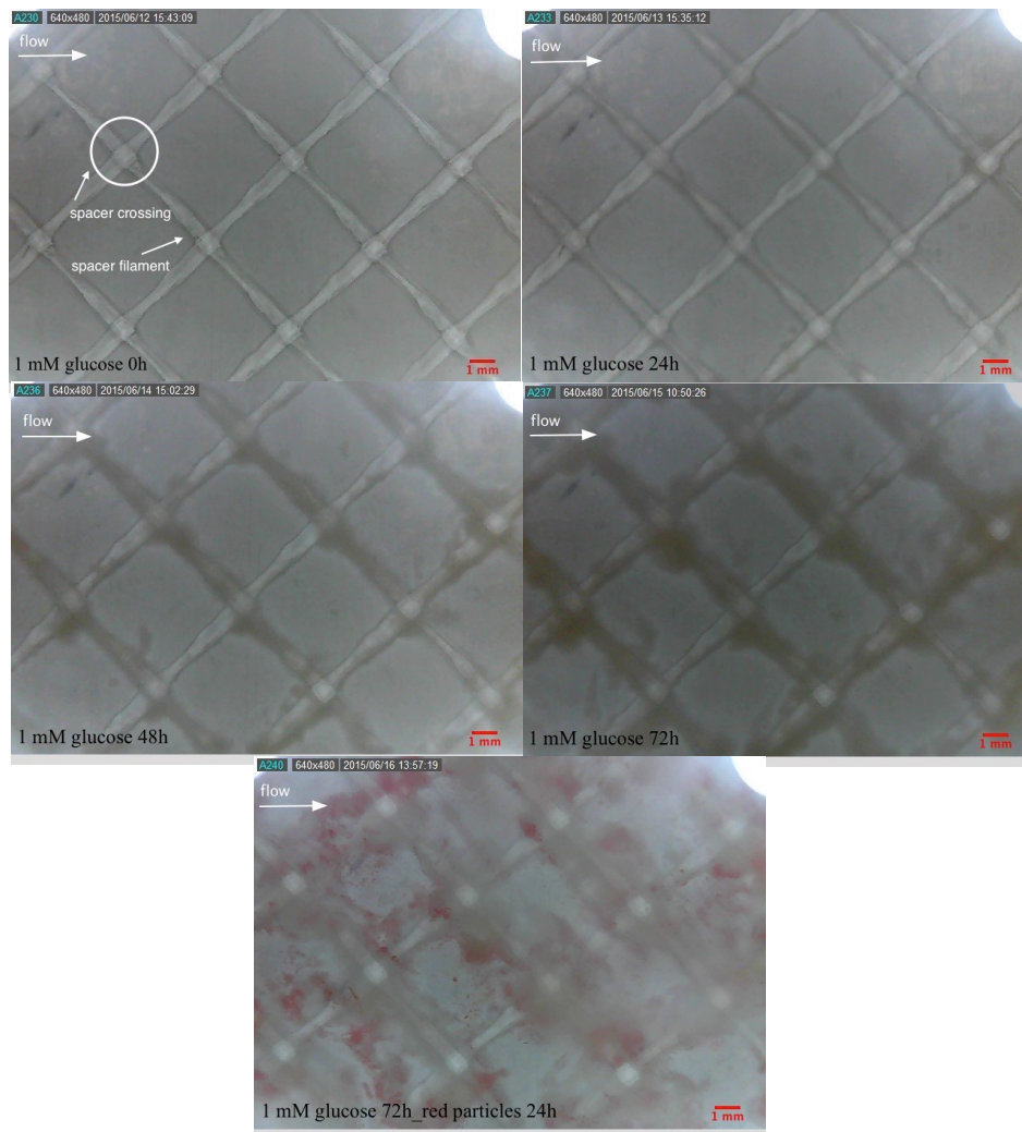
Figure 3. 6 Optical Micrographs of Biofilm Formation during 72-hour Flow of Secondary Effluent Water with 1.0 mM Glucose Followed by 24-hour Flow of Red Dyed Microsphere Particles.
