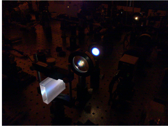
Figure 13. White light are emitted by focusing the creation laser in the quartz cell filled with water.
