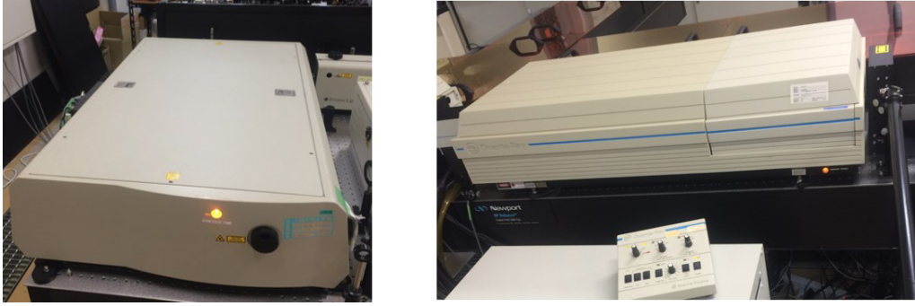
Figure 12. The pictures of the creation laser (left: Hurricane, manufactured by Spectra-Physics) and the inducing laser (right: GCR350, manufactured by Spectra-Physics).
