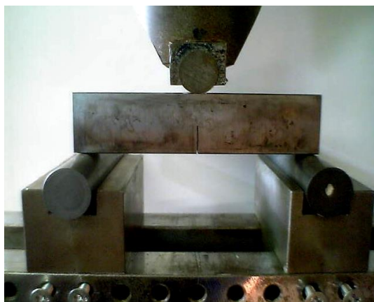
Fig. 5.1.1 Fracture test by 3 points bending
