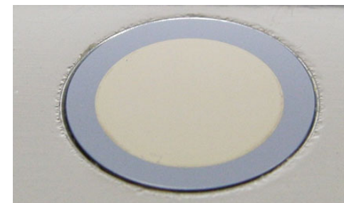
Au surface on Si prism of ATR \sim 8 nm thickness
