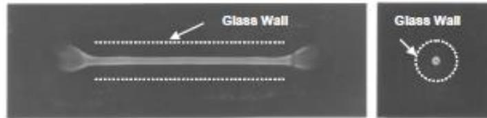
Fig. 1.2 A Swirl type Tubular flame for fundamental study
