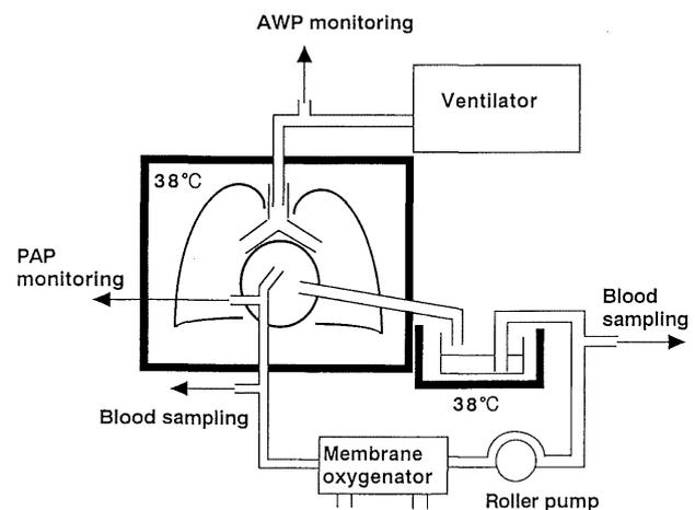
**Fig. 1.** The perfusion circuit.
