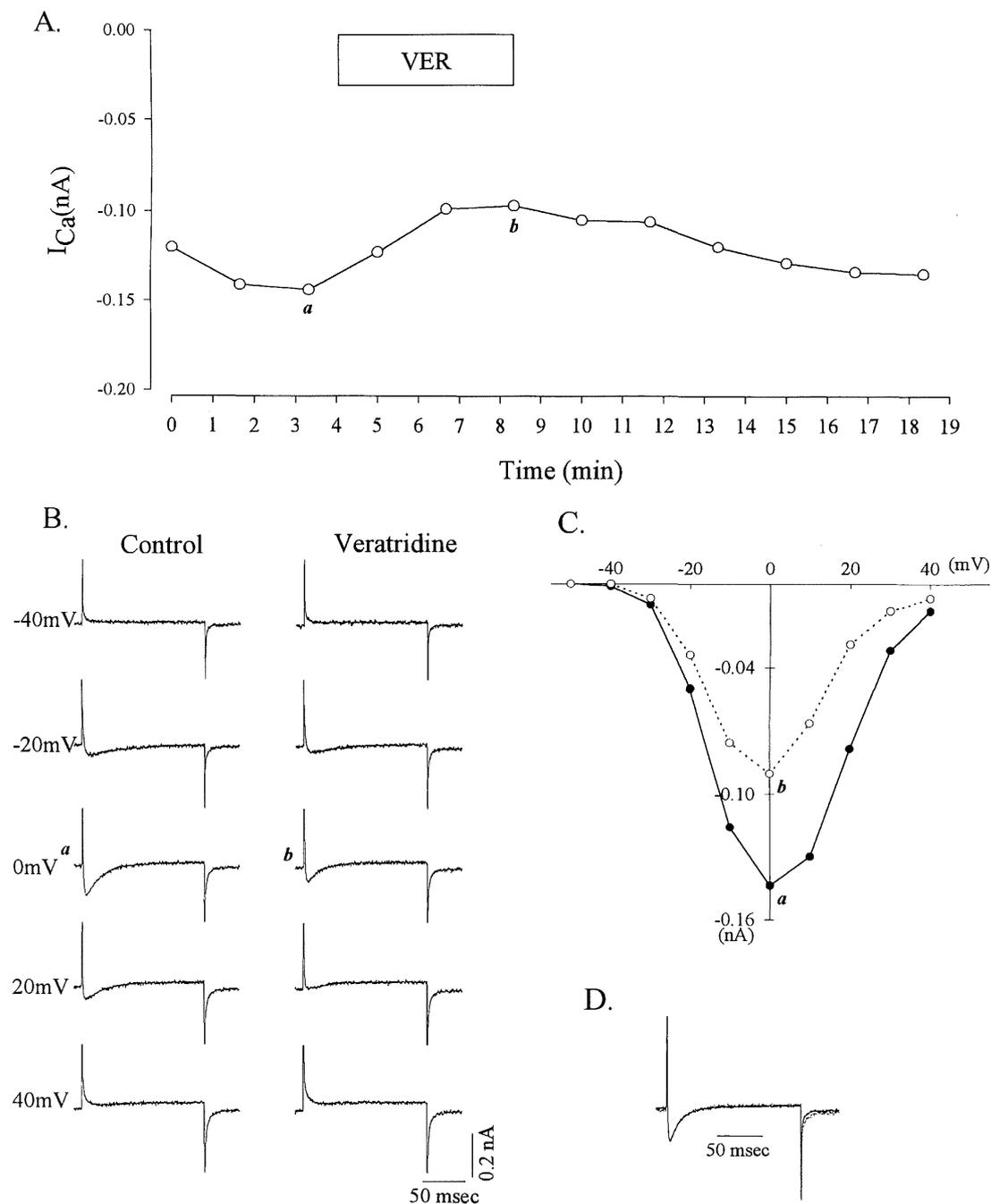
**Fig. 4.** Suppression of  $I_{Ca}$  caused by 100  $\mu$ M veratridine in the external medium.
