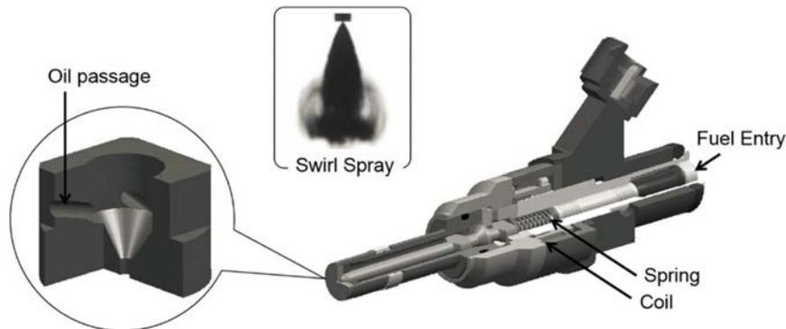
**Figure 1.8** Swirl injector and swirl spray (Kang et al, 2004).
