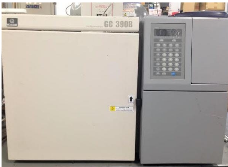
Fig. 4.3. Photographs of GC-390B, GL Sciences.
