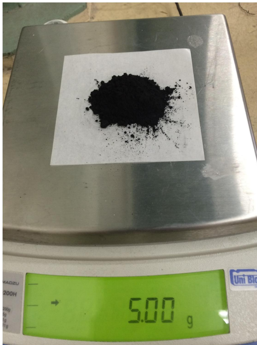
Figure 5.11 Activated carbon powder made from coconut shell with median particle size of 29 \mu\text{m} supplied from PDX-1, Kuraray Co., Ltd..
