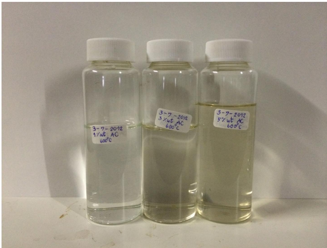
Figure 5.3 Liquid samples of experimental on effect of glycine concentration, reaction temperature of 600 °C, reaction pressure of 25 MPa., and feedstock flow rate of 2 g/min.
