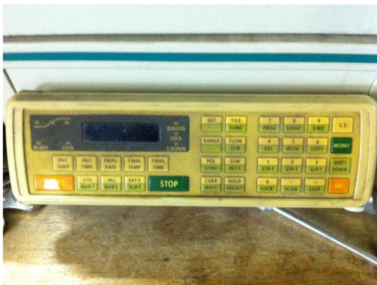
Figure 4.3 GC Control panel
