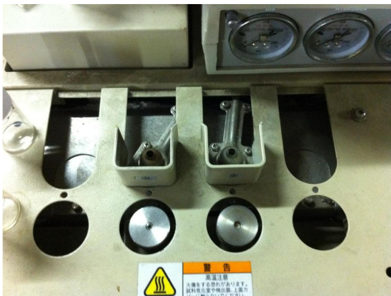
Figure 4.6 Igniters and Injectors
